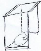
Sketch of proposed shelter, to be constructed of tubular frame with iron covering, with 4 uprights set in concrete.
